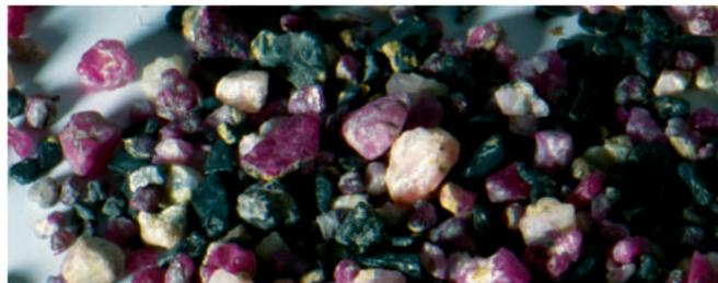
Liberation of coarse corundum from silicate matrix of a metamorphic rock.
