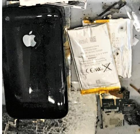
Coarse size processing for liberation of components and batteries
