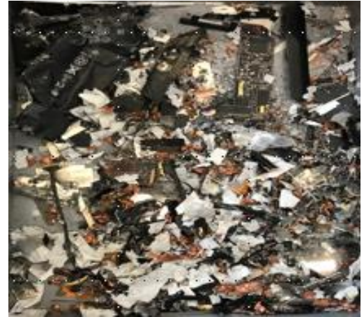
Small size processing for liberation of precious metals & rare earth bearing elements
