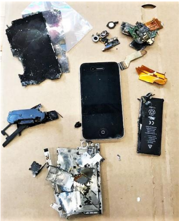
Coarse size processing for liberation of components and batteries
