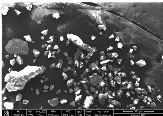
Figure 1 SEM Image of mixed grains of material following dense mineral separation steps.
